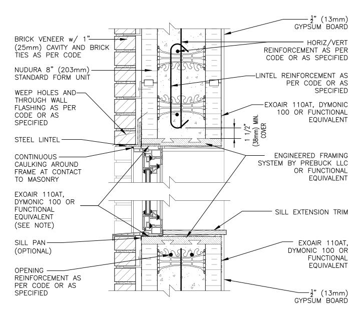
NOTE: AIR BARRIER/DRAINAGE FLASHINGS TO BE INSTALLED AROUND COMPLETE OPENING PERIMETER AS PER SECTION 9.1 OF THE NUDURA INSTALLATION MANUAL OR AS DETAILED BY LOCAL APPLICABLE CODES (CODE GOVERNS)
