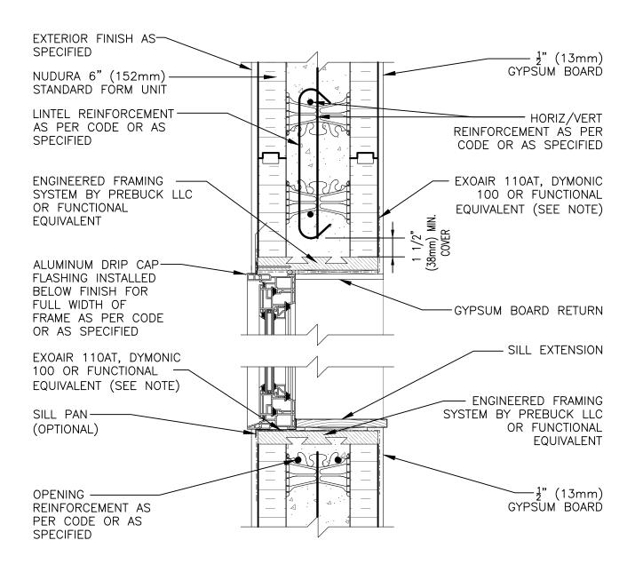
NOTE A: AIR BARRIER/DRAINAGE FLASHINGS TO BE INSTALLED AROUND COMPLETE OPENING PERIMETER AS PER SECTION 9.1 OF THE NUDURA INSTALLATION MANUAL OR AS DETAILED BY LOCAL APPLICABLE CODES (CODE GOVERNS)
