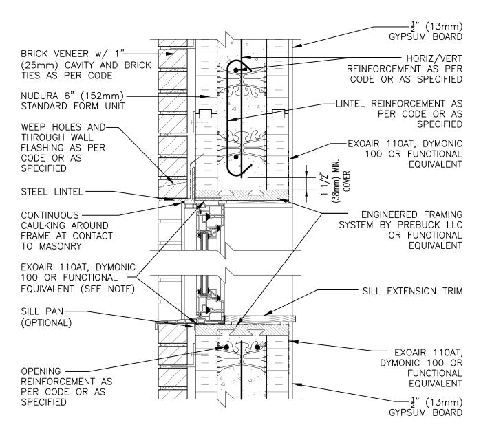
NOTE: AIR BARRIER/DRAINAGE FLASHINGS TO BE INSTALLED AROUND COMPLETE OPENING PERIMETER AS PER SECTION 9.1 OF THE NUDURA INSTALLATION MANUAL OR AS DETAILED BY LOCAL APPLICABLE CODES (CODE GOVERNS)
