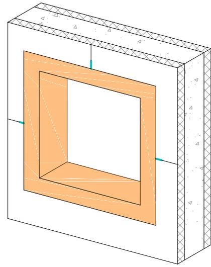
APPLY ENVIRO-DRI 3" MIN INTO ROUGH OPENING AND EXTERIOR FACE OF WALL AT SILL, JAMBS, HEAD
