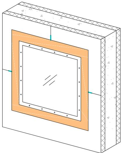
INSTALL NAIL FLANGE WINDOW, SET IN CONTINUOUS BEAD OF DYMONIC 100 EXCLUDING WINDOW SILLS
