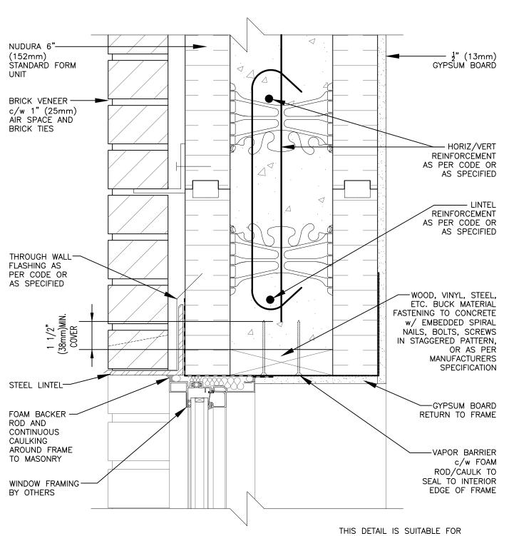
THIS DETAIL IS SUITABLE FOR NON-COMBUSTIBLE 1 TO 3 STOREY HIGH APPLICATIONS AS PERMITTED UNDER LOCAL CODES; FOR WINDOWS IN BRICK CLAD MULTI-STOREY APPLICATIONS, REFER TO DETAIL H6A04 & H6A05 UNDER THIS SECTION
