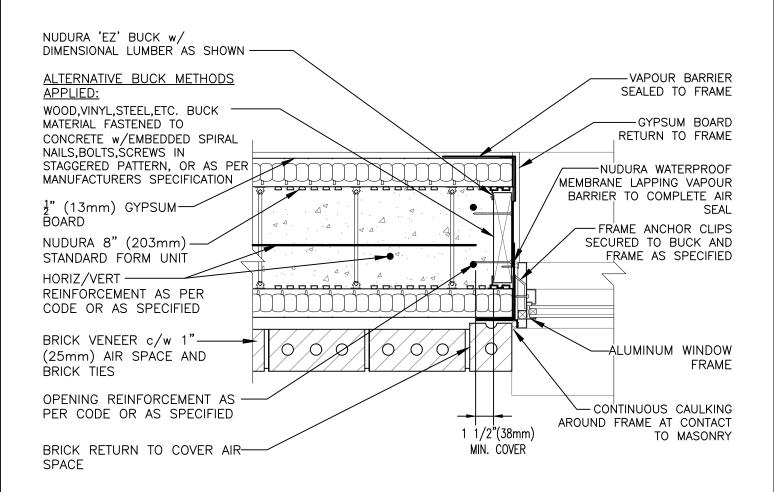
THIS DETAIL IS SUITABLE FOR NON-COMBUSTIBLE 1 TO 3 STOREY HIGH APPLICATIONS AS PERMITTED UNDER LOCAL CODES; FOR WINDOWS IN BRICK CLAD MULTI-STOREY APPLICATIONS, REFER TO DETAIL E8D06 UNDER THIS SECTION
