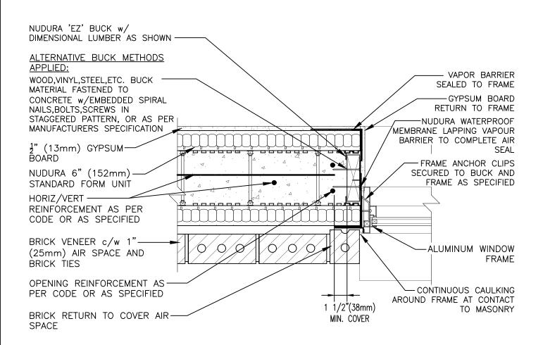
THIS DETAIL IS SUITABLE FOR NON-COMBUSTIBLE 1 TO 3 STOREY HIGH APPLICATIONS AS PERMITTED UNDER LOCAL CODES; FOR WINDOWS IN BRICK CLAD MULTI-STOREY APPLICATIONS, REFER TO DETAIL E6D11 UNDER THIS SECTION
