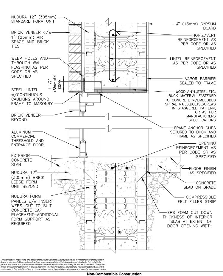
Detail: Nudura 12" (305mm) Form Unit, Wood Buck Mounted Aluminum Entrance Door at Head and Concrete Threshold, Brick Veneer Finish
