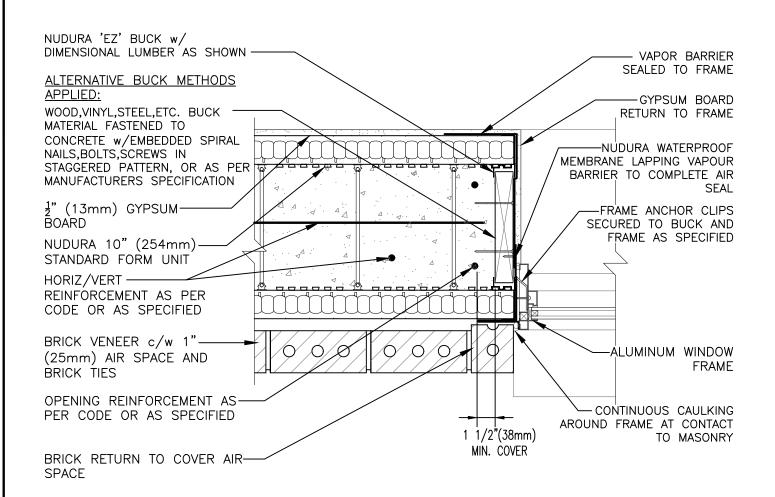
THIS DETAIL IS SUITABLE FOR NON-COMBUSTIBLE 1 TO 3 STOREY HIGH APPLICATIONS AS PERMITTED UNDER LOCAL CODES; FOR WINDOWS IN BRICK CLAD MULTI-STOREY APPLICATIONS, REFER TO DETAIL E10D06 UNDER THIS SECTION
