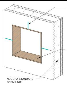
VERTICAL AND HORIZONTAL SEAMS MUST BE DETAILED WITH DYMONIC 100 FROM EDGE OF OPENING AND EXTEND BEYOND FLASHING MATERIALS BY 1" MINIMUM; VERTICAL SEAMS REQUIRE THE DYMONIC 100 TO GO BACK TO CONCRETE FACE AND FILL VERTICAL SEAM
