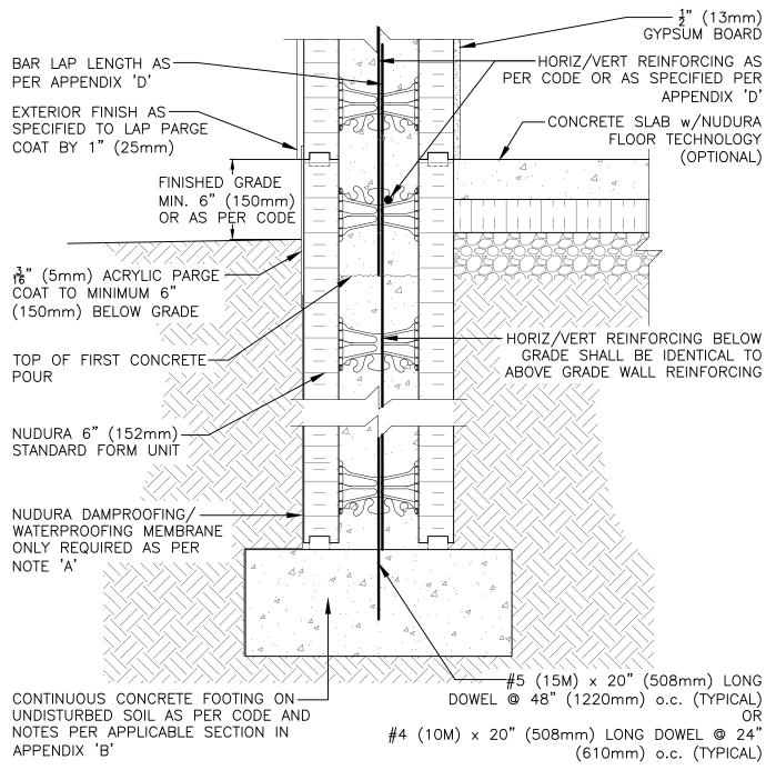
NOTE A: NUDURA DAMPROOFING/WATERPROOFING MEMBRANE IS  $\underline{\text{NOT}}$  REQUIRED EXCEPT WHEN THE INTERIOR FINISHED FLOOR LEVEL IS BELOW THE EXTERIOR FINISHED GRADE LEVEL
