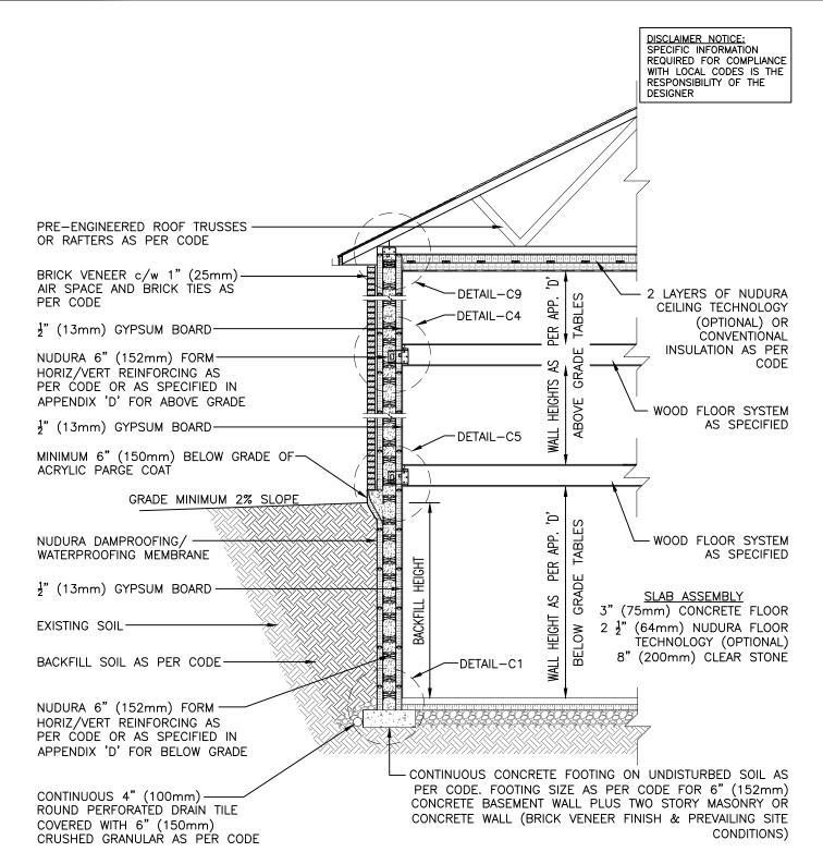
\*NOTE: IN ADDITION TO FOOTING SIZE INDICATED BY CODE, ADD 1" (25.4mm) WIDTH TO STRIP FOOTING FOR EVERY 1'0" (305mm) OF CONCRETE WALL HEIGHT ABOVE 8'0" (2440mm) PER STORY
