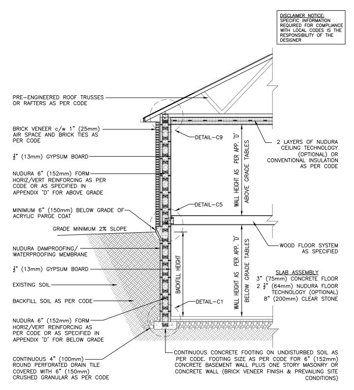
\*NOTE: IN ADDITION TO THE FOOTING SIZE INDICATED BY CODE, ADD 1" (25.4mm) WIDTH TO STRIP FOOTING FOR EVERY 1'0" (305mm) OF CONCRETE WALL HEIGHT ABOVE 8'0" (2440mm) PER STORY
