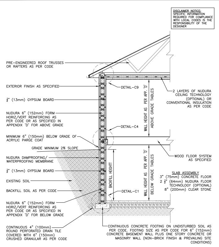
\*NOTE: IN ADDITION TO FOOTING SIZE INDICATED BY CODE, ADD 1" (25.4mm) WIDTH TO STRIP FOOTING FOR EVERY 1'0" (305mm) OF CONCRETE WALL HEIGHT ABOVE 8'0" (2440mm)
